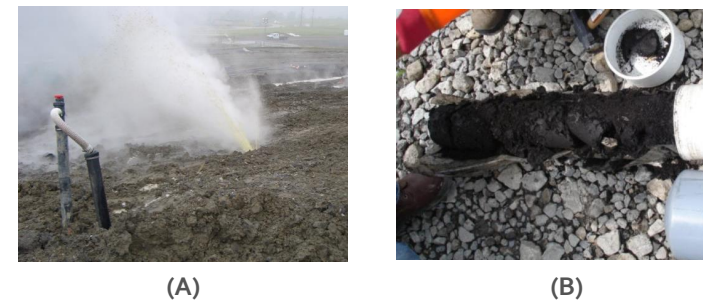
Figure 2. Photos of: (a) leachate geyser of 2 to 4 m high from MSW landfill side slope, and (b) Thermally degraded (combusted) waste from 100 mm diameter rotonomic sample
