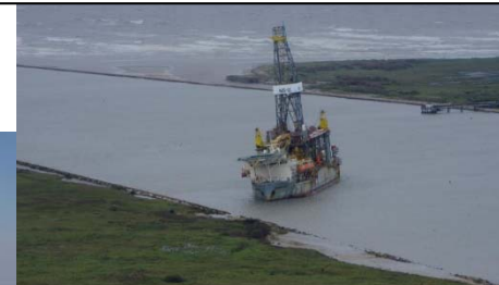
Listing drilling rig (Port Aransas)
